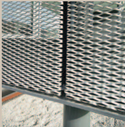
Project: Dachtler Partner AG (CH) - Mesh: Fils 5 - DL 62.5 x DC 20 (20) - av 7.5 x sp 1.5 mm Natural aluminium - Photo: Huber
