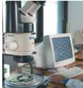
Dimensional control of the apertures in expanded mesh using microscopes and electronic means
