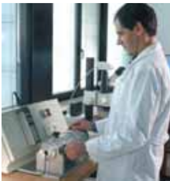
Laboratory equipment for checking the aperture percentage in expanded mesh
